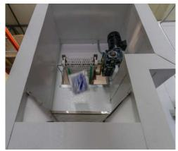
A box of chain-linked bags filled with a freezing compound is placed at the head of the freezer The bags are fed into a water injection system that opens, fills, reseals and separates them to be introduced to the freezer.
